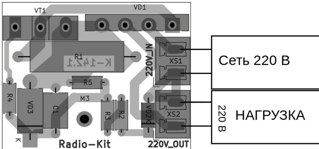
**IMPORTANT!** The whole circuit does not have galvanic isolation with a 220V network, so be extremely ATTENTIVE, avoid touching the board and parts on it during its operation!
